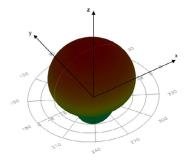
\*Radiation pattern of a single antenna. In the system antennas are installed over metal plate, which eliminates back lobe radiation.
