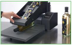
With the built-in LED display users can easily set-up variable spacings, save up to nine different container offsets and see the number of applied labels.
